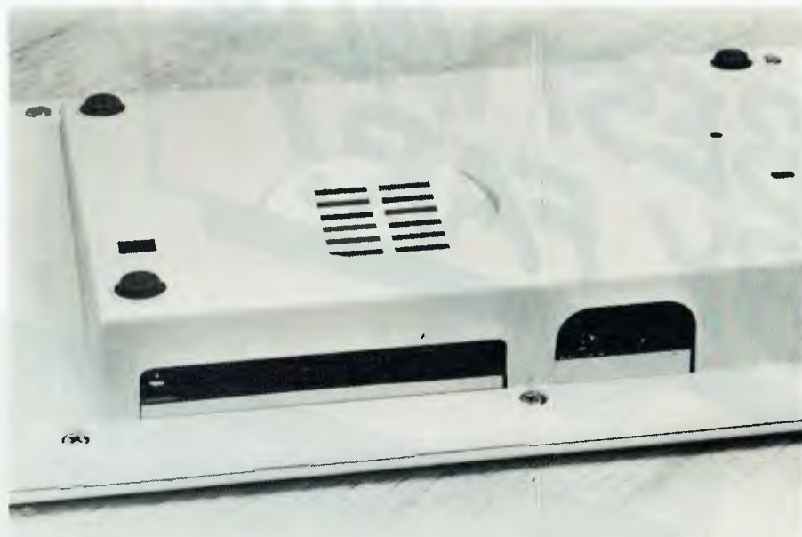
A view of the underside of the Oric, showing its expansion slots at the back.
