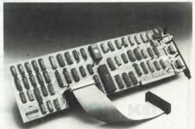
The Quadlink board installs in an IBM-PC, giving it the ability to run Apple programs.
